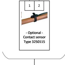
for switching H/K in 2-pipe systems. Only in conjunction with a 3-way valve!
