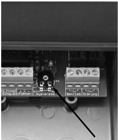
Fig. 4: Setting the differential gap
