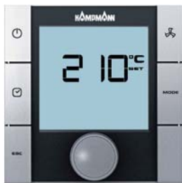
Parameter P36 = 0 "absolute" setting of setpoint temperature
