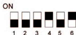
DIP switch factory setting Venkon AC/EC 2-pipe Control configuration -EC1
