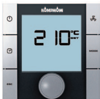
Parameter P36=0 Setting of "absolute" setpoint temperature
