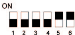
DIP switch factory setting Venkon AC/EC 4-pipe Control configuration -C1
